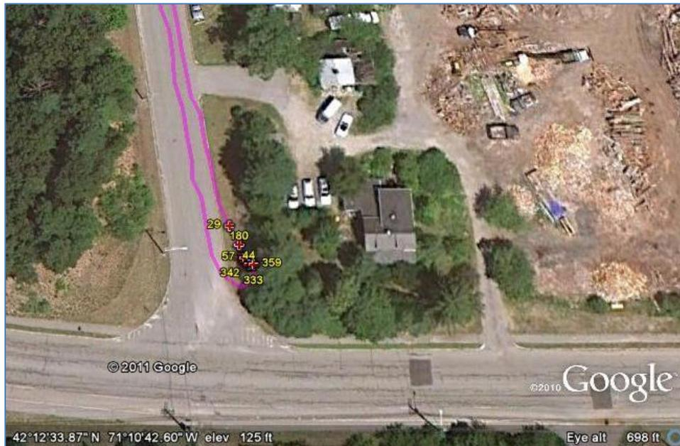
The surveyor’s path is marked in purple and leaks are marked with red crosses. Many times, leaks are stacked on top of one another. To expand any leak readings, place the
