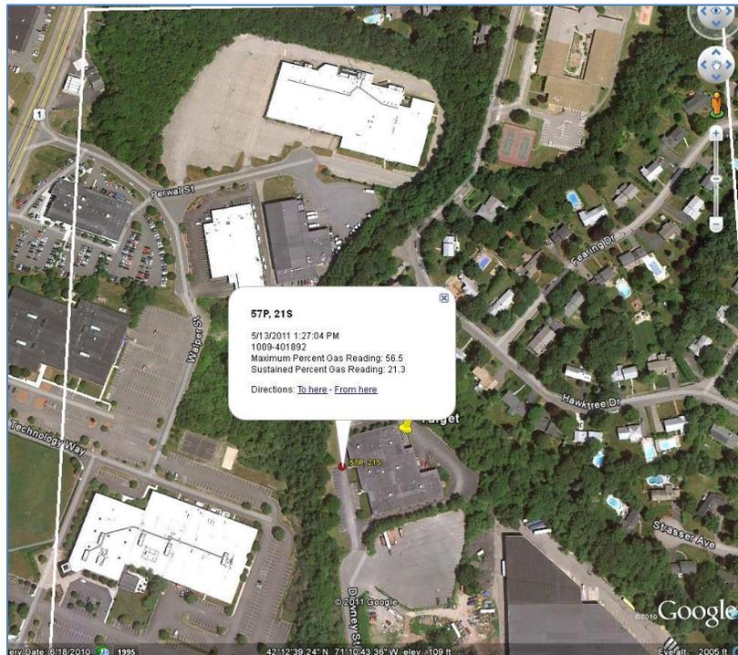
Bar holes with gas readings are marked in red, bar-holes with no gas readings are marked in black. Bar-Holes are usually stacked on top of each other. To expand a set of bar-holes, place the cursor over the set until the white hand transforms to a cross, click to expand. To select detailed readings for a single bar hole, expand any bar holes with the cross and then select an individual bar hole with the cursor.
